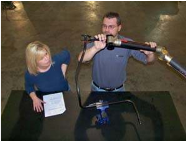
Traci Kramer (left) and Josh Hairell of Harco use a Romer CimCore laser tube inspection system to inspect tube geometry.
